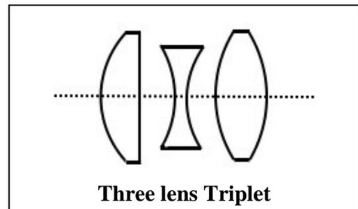
Before you purchase a 10X loupe you should test it to see that both the chromatic and spherical distortions have been eliminated. You can test your loupe for chromatic aberration by looking at a white light source through your loupe. If the image remains white (also on the outer edge) it will be achromatic. Spherical aberration can be tested on squared drawing paper. The squares should remain square in the total view of your loupe.
