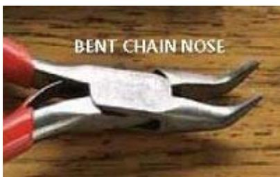
**Bent-nose (or bent chain-nose) pliers** are wire jewelry expert (and *Step-by-Step Wire Jewelry* magazine editor) Denise Peck's favorites. "The best tip I ever learned in jewelry school was to use two bent-nose pliers for opening and closing jump rings. Bent-nose pliers allow you to firmly grasp both sides of the ring without obscuring the opening from view."
