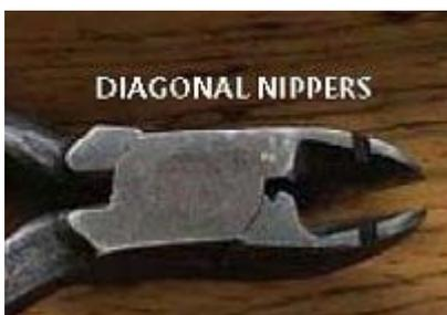
**Cutters (or nippers)** are pliers with a cutting edge that may be on the side or at the end of their jaws. The cutting edge may sever wire cleanly (as with flush cutters) so that one or both wire ends are flat, for a smooth fit, or they may simply cut wire, leaving a small peak or point where the wire was pinched during cutting.
