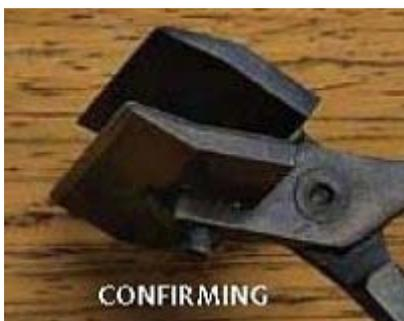
**Confirming pliers** are mostly for working with (or creating) corrugated metals. Their edges are thin, flat, and wide, making them ideal for pinching or "confirming" edges of metal folds. Tip: I also find them handy to hold a wider strip of metal when I'm texturing or stamping on it, rather than using regular pliers (which can leave marks around where their skinny jaws grip the metal) or my fingers (which can get whacked!).
