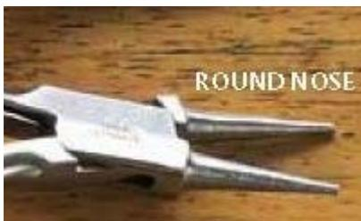
**Round-nose pliers** have round jaws that taper from their point to their broader base. They're ideal for making loops, coils, and curved bends. (Tip: To make consistently sized loops for a project or when making lots of eye pins, mark the jaws with a marker and make all your loops on that line.)
