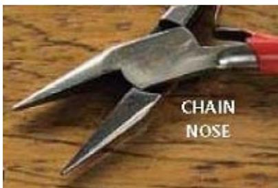
**Chain-nose pliers** usually have tapered jaws that are flat inside and half round on the outside. Their jaws may be extra long or curved. They're ideal for loops and curves with a small radius.
